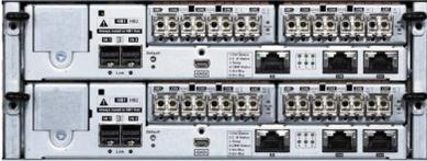
Universal ports accept SFPs for 8 Gb & 16 Gb Fibre Channel and 10 Gb Ethernet that support simultaneous multi-protocol access. Protocols are easily changed with SFP swaps.
